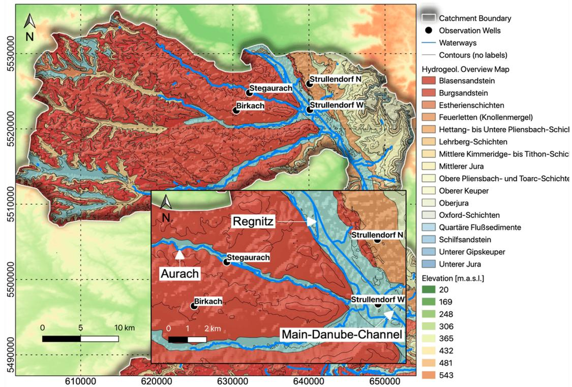
**Figure 6:** Subordinate catchment in the center of the Main catchment in central Germany. Topography is indicated with black line (no labels) and the geology with colored layers. Bottom, right: Zoom closer to the four investigated groundwater observation wells and the valley with the Regnitz river.
