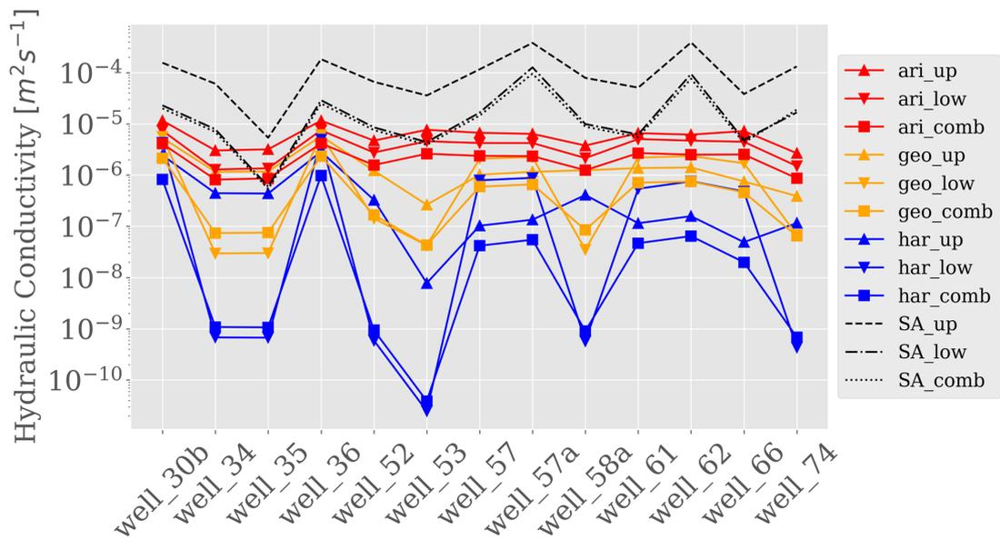
**Figure 21:** Results of the spectral analysis using thicknesses of only upper (SA\_up), lower (SA\_low) and combined (SA\_comb) layers for every well and weighted, averaged hydraulic conductivities for each slice.
