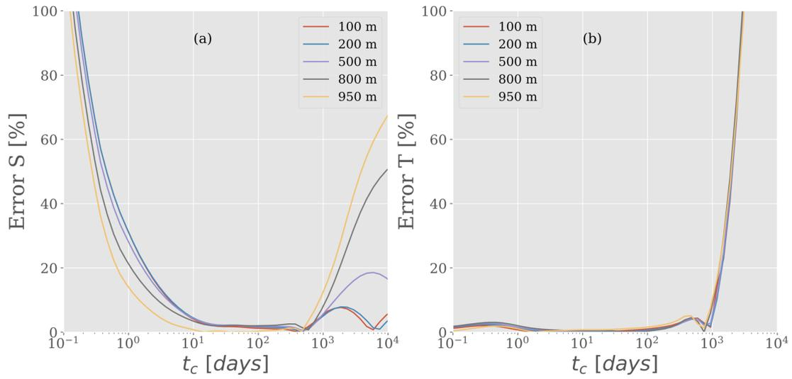
**Figure 3:** Error of deviation between input (numerical model) and output (spectral analysis) aquifer parameters with respect to input parameters plotted against the characteristic time  $t_c$  of the aquifer for five locations. (a) Error of storativity. (b) Error of transmissivity.
