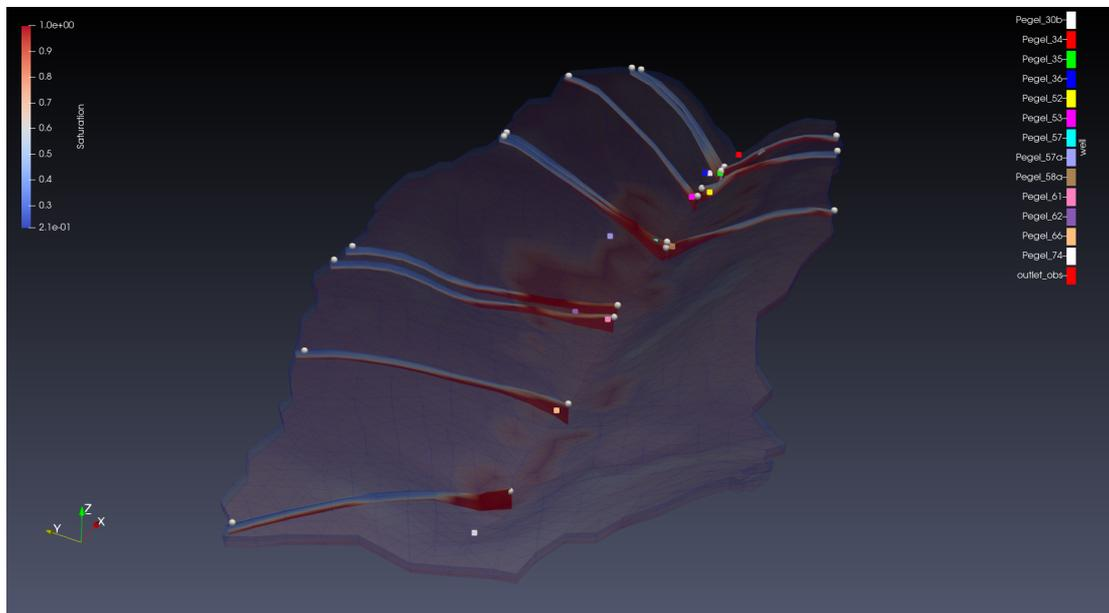
**Figure 22:** Modeling domain (transparent) and slices with saturation for a single day. Towards the center of the catchment the saturation increases.
