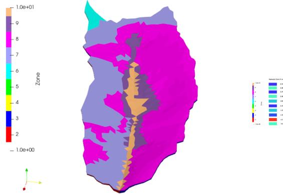
**Figure 17:** Slicing the numerical model. Each zone was parameterized with another hydraulic conductivity (see legend on the right).
