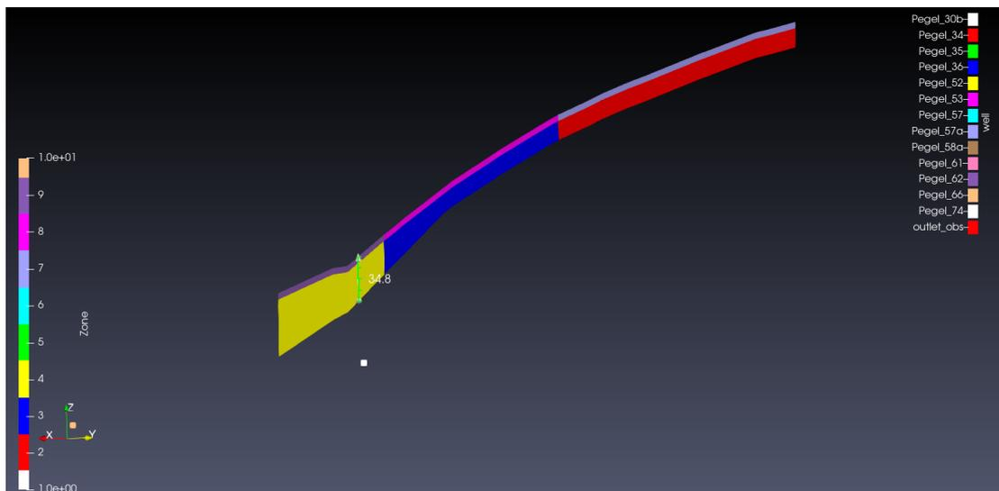
**Figure 19:** A single slice wich corresponds to observation well 30b. The thickness  $b$  at the location of the observation well has been estimated to calculate the hydraulic conductivity  $K$  from the derived transmissivity  $T$  by the spectral analysis with  $K = T / b$ .
