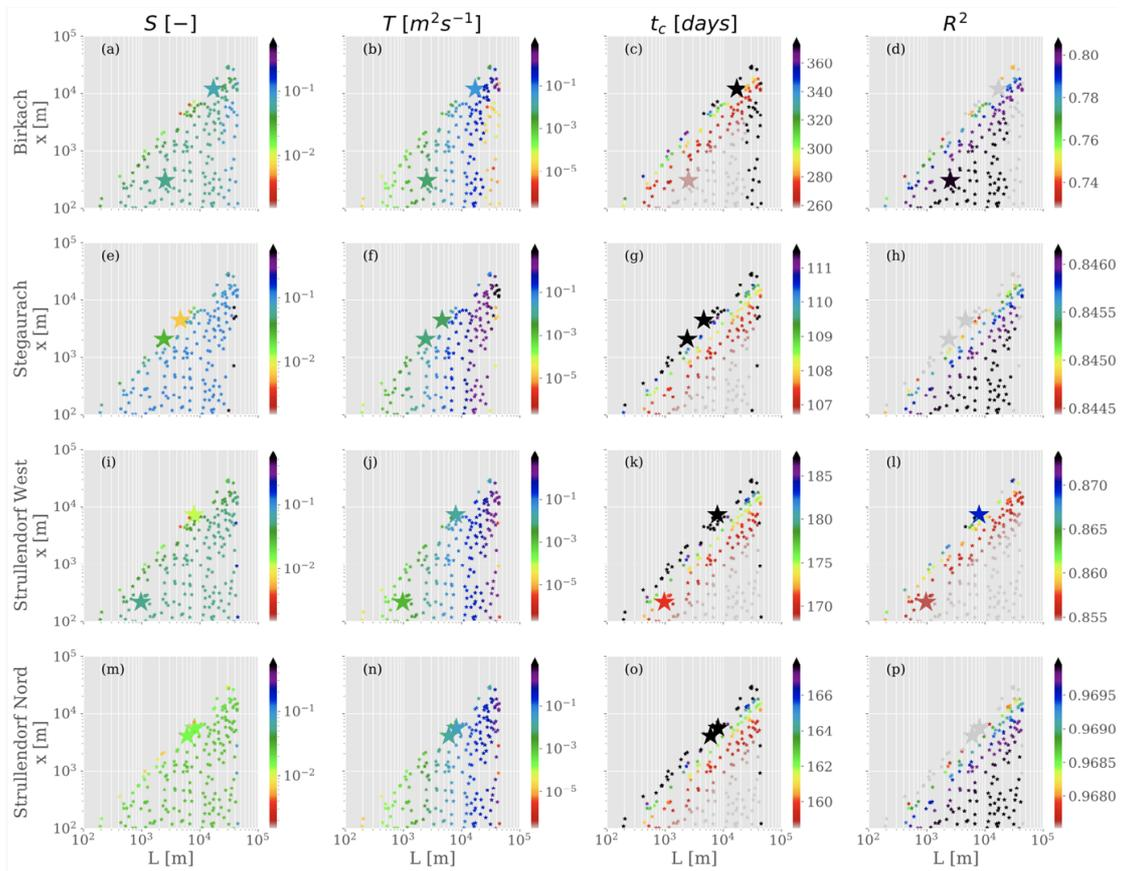
**Figure 9:** Scatter plots of derived storativity  $S$ , transmissivity  $T$ , and resulting characteristic time  $t_c$  for different combinations of aquifer length  $L$  and distance to water divide  $x$ . The goodness of the fit was evaluated with the  $R^2$  value. Color bars of  $S$  and  $T$  have the same log-scale for every observation point, whereas the linear scale for  $t_c$  and  $R^2$  was adjusted in each plot. The big stars represent the manually added samples.
