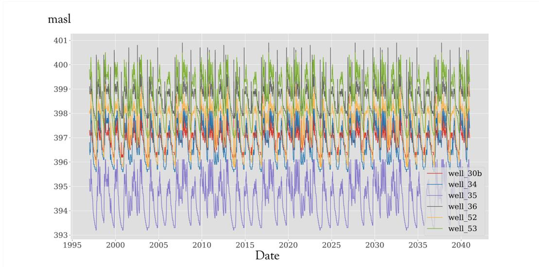
**Figure 13:** Groundwater level fluctuations for observation wells 30b, 34, 35, 36, 52 and 53.
