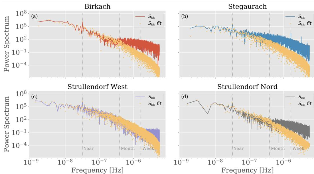
**Figure 10:** Spectra of groundwater heads ( $S_{hh}$ , solid) and a corresponding fit of the analytical solution ( $S_{hh}$  fit, dots) with the best  $R^2$  value, selected from the two manually added samples.
