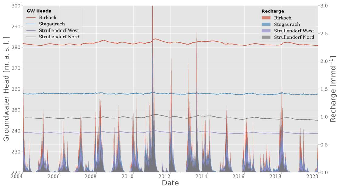
**Figure 7:** Groundwater head time series of four observation wells in the central Main catchment and corresponding recharge modeled with mHM.
