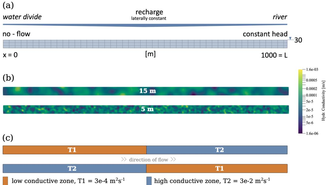
**Figure 2:** (a) Aquifer geometry, forcing and boundary conditions for all setups (b) One realization of each correlation length of an isotropic, log-normal distributed hydraulic conductivity field generated from a Gaussian covariance model with variance 1. Top: 15 m, bottom: 5 m correlation length. (c) Deterministic block aquifer with two zones of hydraulic conductivity. The position of the boundary between the zones was varied throughout the investigation.
