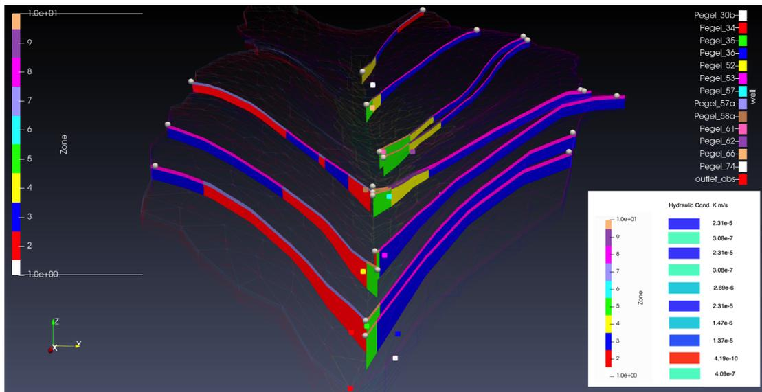
**Figure 18:** Slices of the numerical model which correspond to the transects of the respective wells (scaled in Z with factor 10). Wells are depicted with a colored square (see legend on top right).
