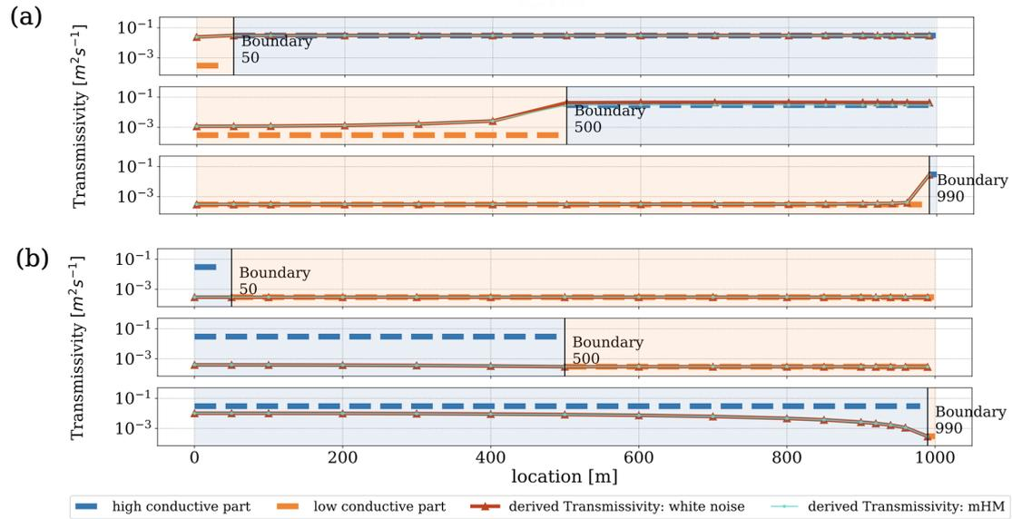
**Figure 5:** Input (numerical model) and output (spectral analysis) transmissivity for six different deterministic aquifers. A white noise and a realistic, temporally correlated recharge generated by mHM was assigned to the numerical model. a) A low conductive zone in the upstream part of the aquifer and a high conductive zone at the outlet b) A high conductive part upstream and a low conductive part downstream.
