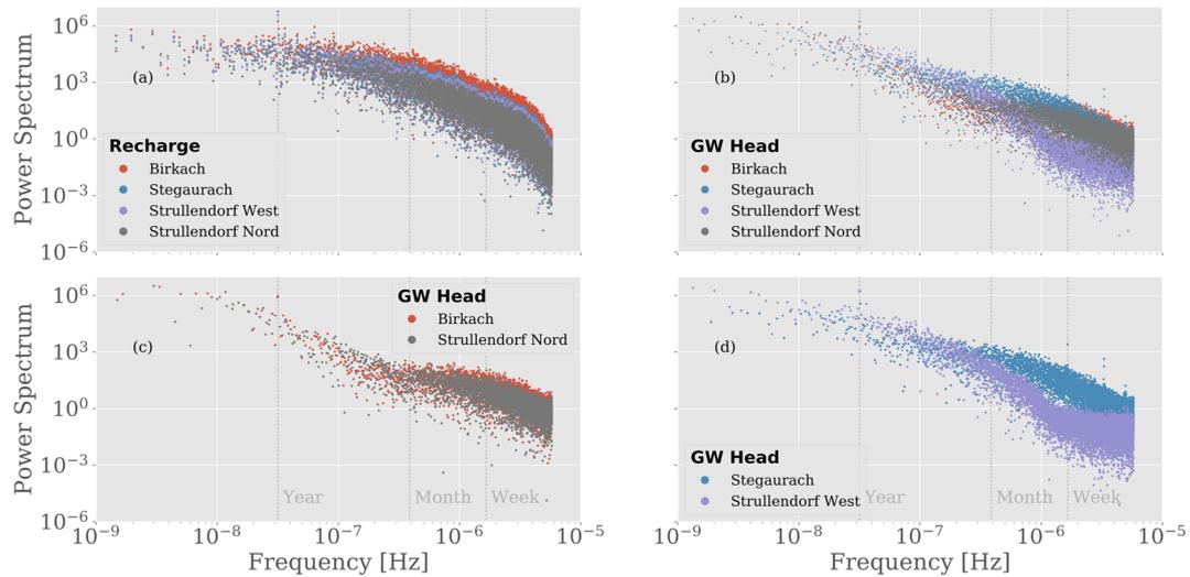
**Figure 8:** Power spectra of recharge (a) and groundwater head time series (b) for each observation well. For a better view, geologically similar wells are plotted in one figure: (c) Screened in Burg- und Blasensandstein, (d) screened in quaternary sediments.
